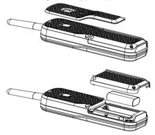
2. Replace the battery cover and screw the cover into place. Finally, screw the belt clip on.
