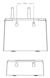
Insert the wall plugs if necessary, then insert the screws leaving about 5mm protruding from the wall on which to hang the phone.
