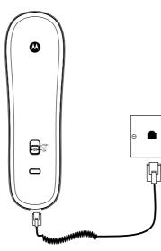
1. Plug one end of the curly line cord into the socket on the handset and the other end into the telephone wall socket.
